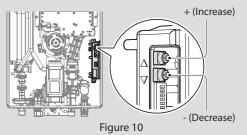
11. When the pressure setting is completed, press the reset button twice to change to <Normal operation mode>.
