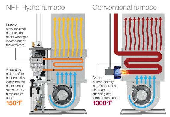
Our unique hydronic forced-air heating design keeps combustion in a separate, fully enclosed compartment for safe and quiet comfort.
