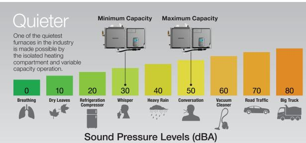
We test our products in a sound laboratory specifically built to resemble a typical residence. Sound level recordings produced at steady state minimum and maximum operation measured three feet from the furnace. Additional sound level information available at: www.ensafe.com/occupational-noise-exposure-key-osha-provisions.
