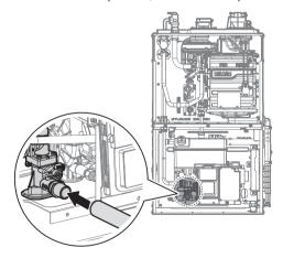
Rotate the drain valve on the drain adapter 90 degrees in a clockwise direction, and then lift up the lever on the pressure relief valve to open it.
