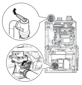
Drain the expansion tank for more than 5 minutes and then close the drain valve and pressure relief valve.
