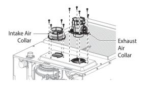
3. Insert the intake filter at the bottom of the intake air collar.
