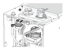
4. Connect the exhaust collar's connector to the VID sensor connector inside the furnace.
