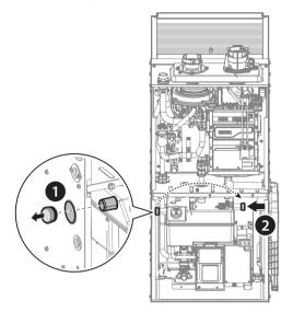
6. Install the left drain trap assembly, junction box, and supply water assembly that were separated as shown in the figure below.
