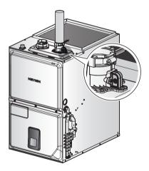
As shown, the VID is a device integral to the vent collar which detects whether the vent pipe has been inserted to a sufficient depth during its installation.
