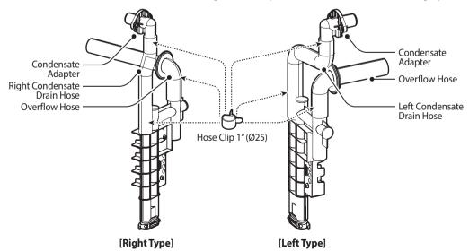
5. Before installing the drain trap assembly on the left side, disconnect the plug installed on the left overflow outlet of the tank and reinstall it on the right side overflow outlet.
