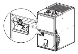
4. Fill with water through the water inlet and Check the water fill level on the front control panel.
