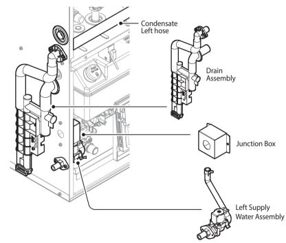
7. When the furnace is commissioned and running, make sure there are no leaks in the hose connections.
