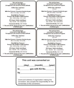
Figure 11. Proper Placement of Gas Conversion Labels
