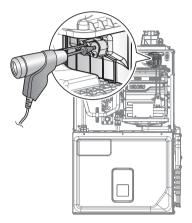
Figure 7. Insert the Analyzer
