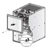
8. Loosen the screws indicated in the figure below and connect a manometer to the pressure port. Reset the manometer to zero before use.
