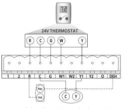
Dehumidistat **Remote Condensing Unit** (Single-Stage Cooling) (Optional)
