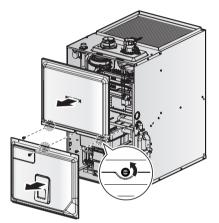
2. Connect the <sup>3</sup>/<sub>4</sub>" condensate hose (included in the installation parts kit) to the drain adapter.
