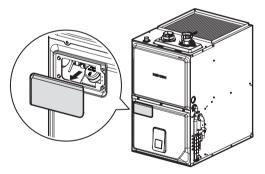
3. Remove the water inlet plug.
